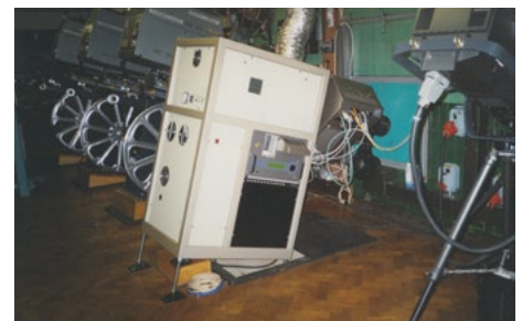
Barco DP50 projector on Kinton console at the Odeon Leicester Square next to three Cinemeccanica Victoria 8s for running both 35mm and 70mm film.
